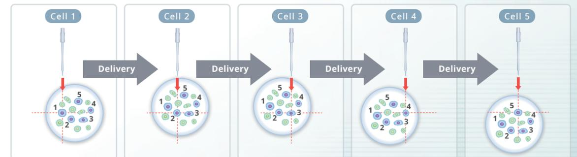
Continuous delivery to multiple cells is possible by connecting the SU10 to the motorized stage of the microscope via external trigger linkage.
