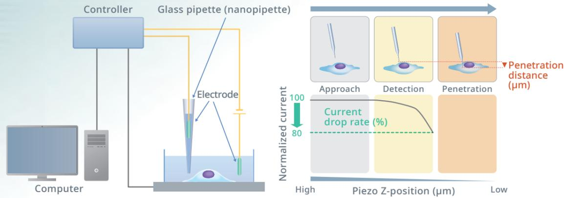
\*A scanning Ion Conductance Microscope: acquires the surface 3D shape of a material by utilizing the decrease in ion current value that occurs as the distance between the probe (glass pipette) and the sample (cells, etc.) gets closer. The SU10 does not have an image acquisition function.
