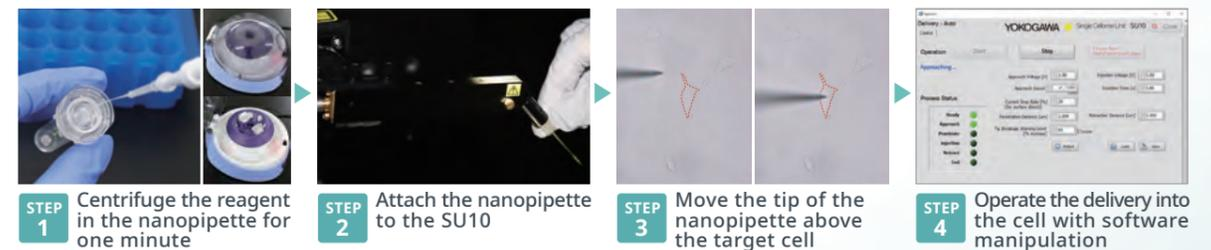
Continuous automatic nano-point delivery including XY positioning of cells
