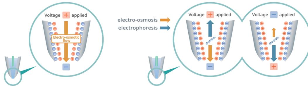
Since the inner wall of the nanopipette is negatively charged, cations and other ions in the liquid inside the nanopipette form an ionic layer. The ionic layer moves toward the tip of the nanopipette when a higher voltage is applied than at the time of approach. The movement of the ionic layer causes the liquid in the nanopipette to move (electro-osmotic flow) and is injected into the cell.
