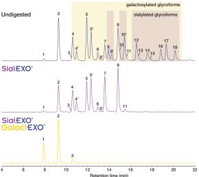
Figure 3. HILIC-FLD UHPLC chromatograms of a 2-AB labeled glycan library analyzed undigested (top), after treatment with SialEXO (middle) or both SialEXO and GalactEXO (bottom). Analysis was performed on a Thermo Scientific Vanquish Duo UHPLC system equipped with a Thermo Scientific Accurcore 150 Amide HILIC column (2.1 x 150 mm).
