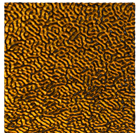
Topography (left) and phase image (right) of an unannealed PS-PB-PS triblock copolymer thin film on mica imaged at 20 Hz line rate using an USC-F1.2-k7.3 cantilever. Image size: 500 nm
