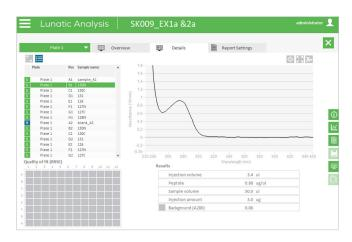
Figure 3: Illustration of the Results screen on the Big Lunatic. In addition to the injection volume, the peptide concentration is also displayed.
