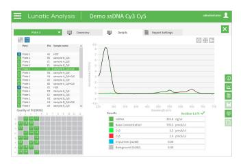
Figure 3: Illustration of the Results screen on the Big Lunatic. Unmix app results of the selected sample are shown as spectral shape as well as in calculated values.
