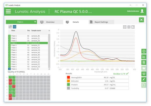
Figure 4: Big Lunatic Analysis software quantifies the plasma-relevant components from the measured UV/Vis absorption spectra.
