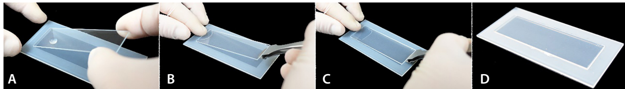
Figure 5-17: Place the scWest chip in the incubation chamber. A: Pipette antibody cocktail solution in a bead on the left side of the incubation chamber. B: Gently lower the chip onto the antibody cocktail. C: Stabilize the scWest chip gel side down using the flat edge of tweezers (without gripping with the tweezers). D: scWest chip incubating in antibody cocktail solution with no air bubbles.
