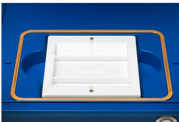
Figure 5-11: Proper seating of the scWest chip and electrophoresis cell inside Milo.
