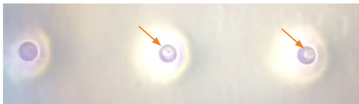
Figure 5-4: Brightfield image of three wells. The well on the left is empty, while the central well and well on the right each contain one cell (arrows).
