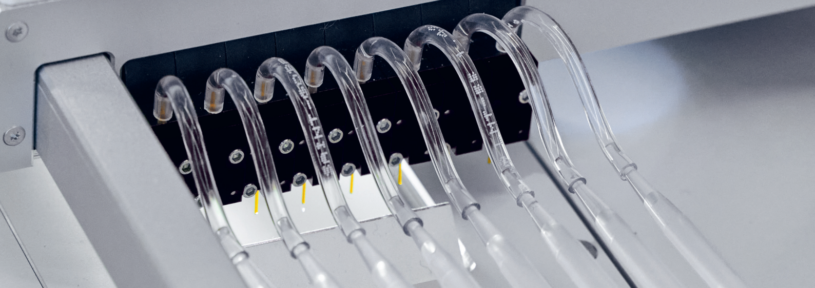
Figure 2. PIPEJET® modules, including pipes (yellow) inside the pipe guides (black), connected to the liquid reservoir tubing
