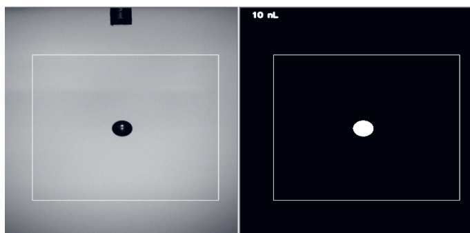
Figure 3. SMARTDROP® technology capturing the drop mid-flight to ensure precise volume calibration across various liquid types.
