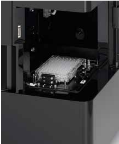
Plate motion uses a fixed probe and moves the plate (and sample) in horizontal and vertical directions.
